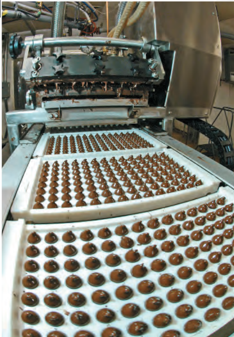
Richard Van Dyke checks the size on chocolate drops being produced on the company's Aasted-Mikroverk one-shot depositing line. The unit can turn out about 6,000 lbs. during an 8-hour shift.
