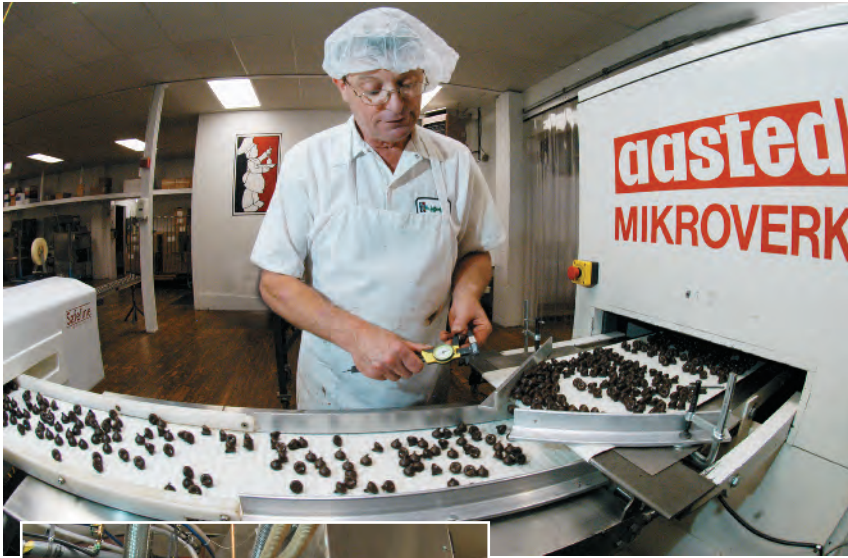
Richard Van Dyke checks the size on chocolate drops being produced on the company's Aasted-Mikroverk one-shot depositing line. The unit can turn out about 6,000 lbs. during an 8-hour shift.
